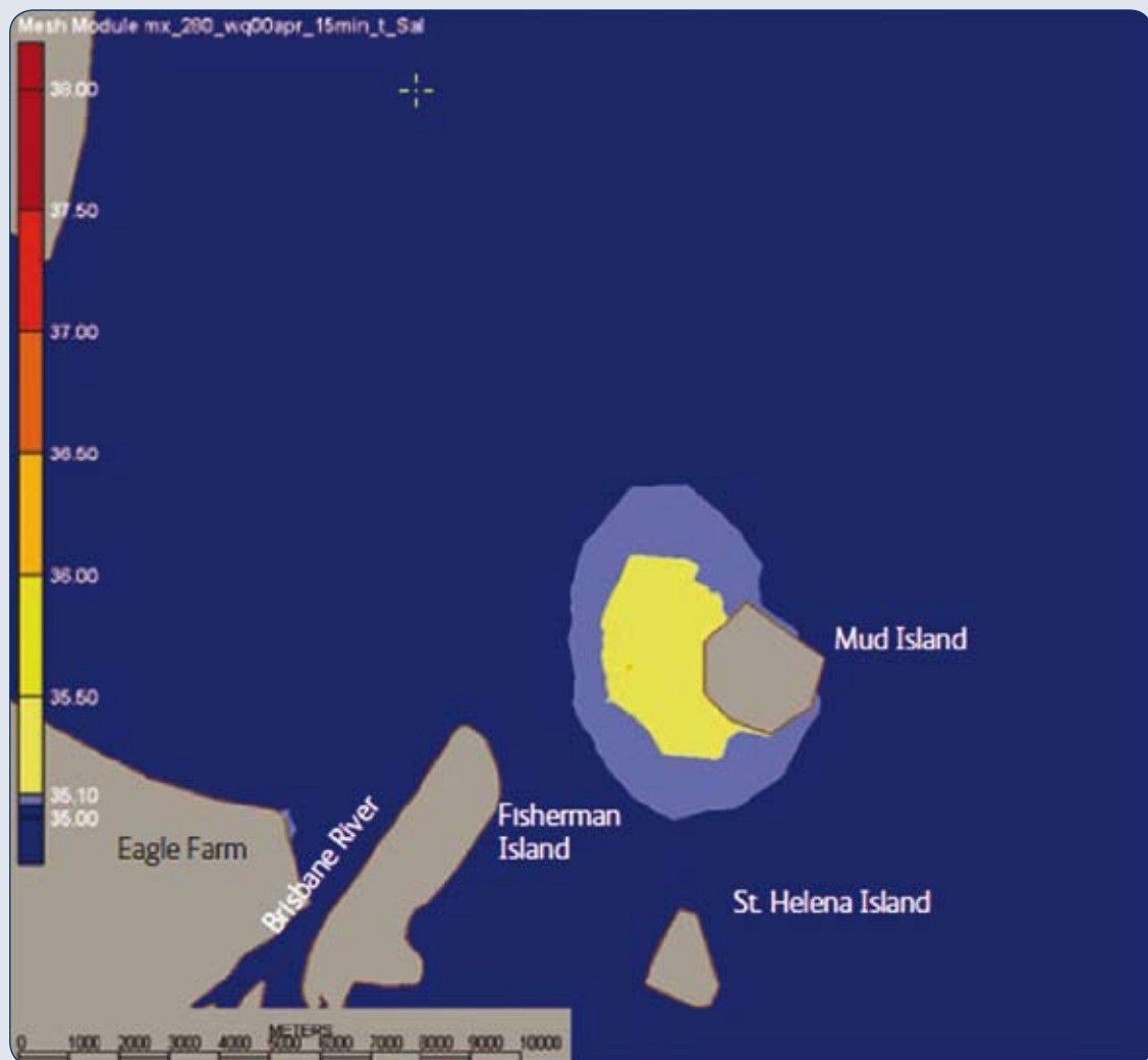
Figure 5.7 Example output from hydrodynamic modelling—median salinity contours
